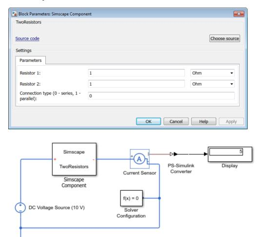
If you change the value of the **Connection type (0 - series, 1 - parallel)** parameter to 1, the resistors are connected in parallel, and the current is 20A.
