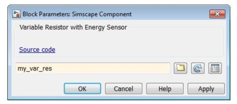
7 Click **OK**. The block icon gets updated, reflecting the selected source component. It now has two conserving electrical ports, + and -, and a physical signal input port PS.
